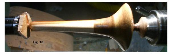
Profile changes (Fig. 10) brought the centre of gravity lower into the bottom but the handle still had too much mass as proven by my tests...it spun for a second or two before toppling over. Testing so far
