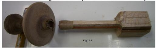
I cut too close to the hole for the handle tenon and the parts separated. Oh well...at least now I know how to approach the design of tops should I want to get into making more of them.
