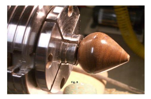
Note (in Fig. 8) that the waste on the bottom's end has been cut away leaving a flat spot the had to be addressed.
