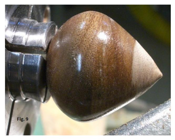
This was done with a sharp skew followed by sanding (Fig. 9 below). Application of finish was done as before. The small cut-off point on the top of each handle was sanded and finished free hand out of the chuck.
