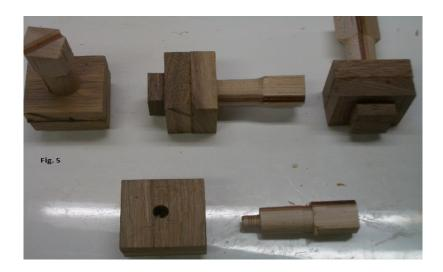
Glue was applied to the tenons, the handles pressed into the bottoms and each placed in a vise for drying (Fig. 6).
