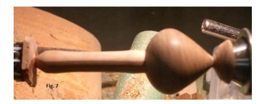
The top was cut free at the handle end with a skew and the handle mounted into the chuck's spigot jaws (Steb centre removed). See Fig. 8. To minimize damage the handle was wrapped with painters' tape before pressure from the jaws was applied. To ensure the whole top was concentric the lathe was turned on and if the point on the bottom showed any wobble the top was repositioned until all wobble was removed.
